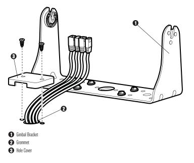
9. Insert cable connectors into the proper recesses on the cable collector insert. The cable connectors are keyed to prevent reverse installation, so be careful not to force the connectors into the wrong slots. If you don't have a cable for every hole in the insert, install the blank plugs to protect the control head from the weather.
